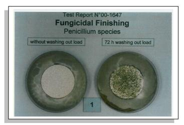
designed to control the growth of fungi and algae on plywood as well as other woods, masonry and other construction materials and coatings.
